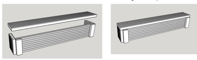
STEP 4 Now turn the window box over and fix the rear section.
