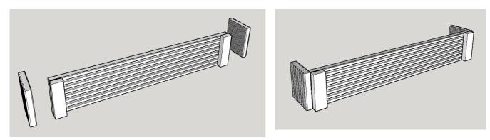
STEP 2 Fix the sides to the floor section using the screws provided making sure the bottom edge of the side is flush with the bottom of the floor section. Note that the sides have pre-drilled holes.
